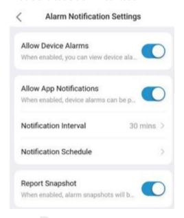
• Tap behind **Receive Alarm Message** to enable or disable alarm notification. After enabling this setting, you also need to enable notification for the app in your mobile phone's system; otherwise, your mobile phone will not receive real-time alarm messages.
